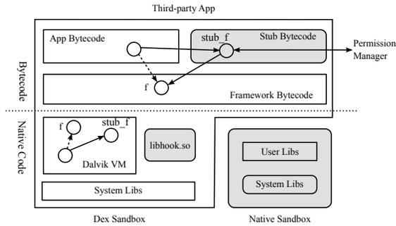
Figure 2: System architecture of AppCage
