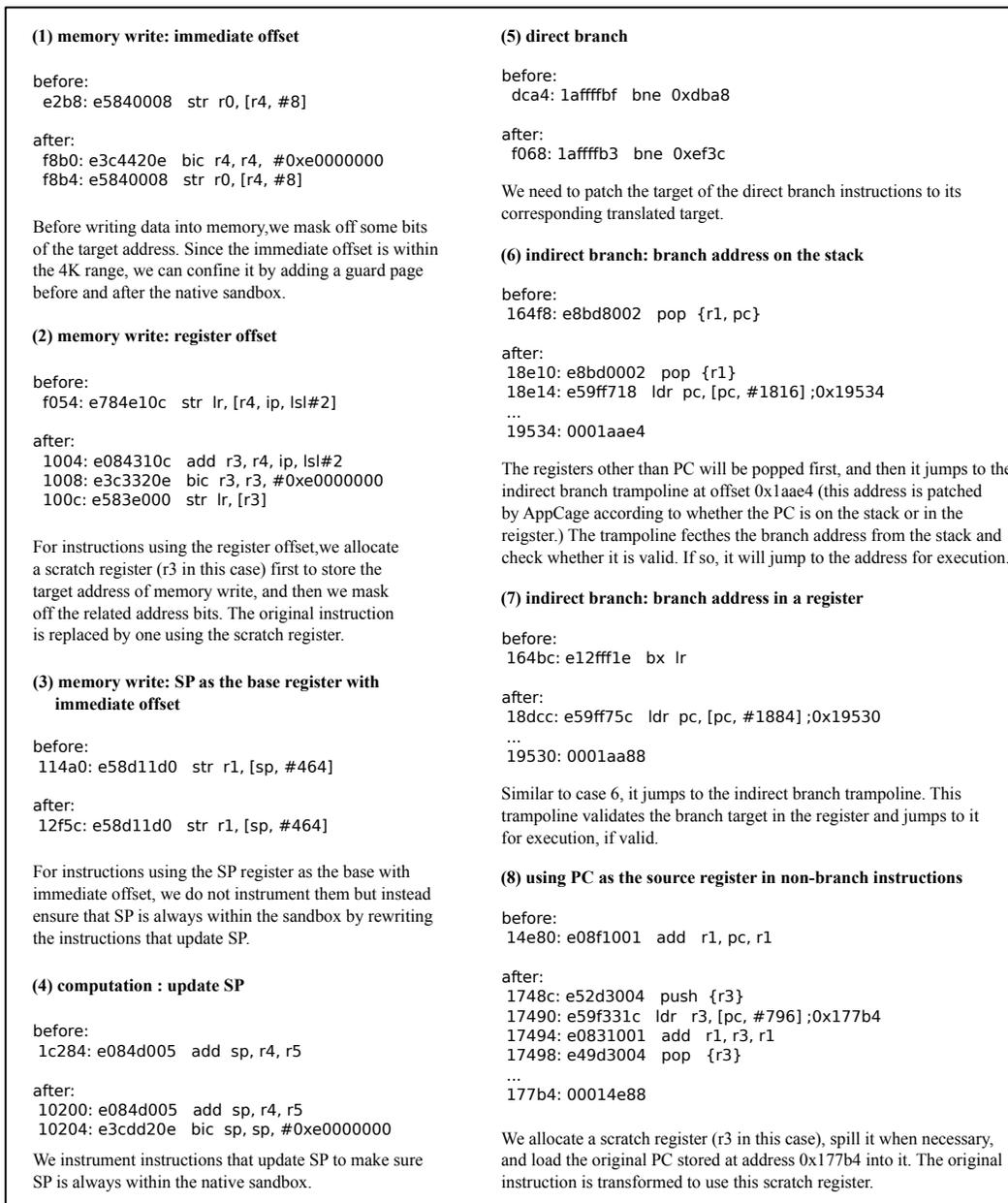
Figure 4: Instrumentation of native code by AppCage
